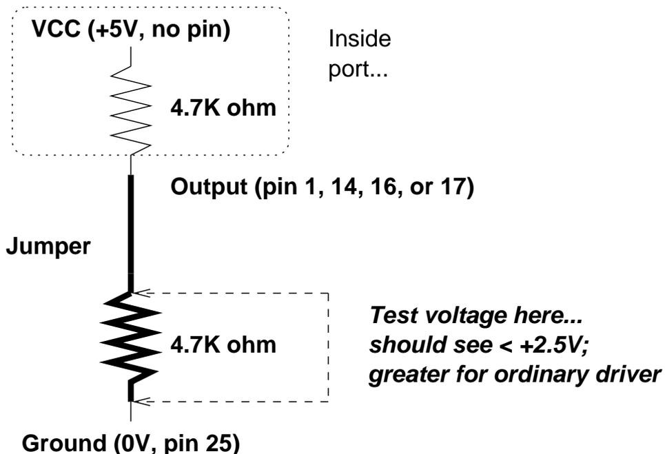
No harm should come to the port hardware in either case, since the 4.7K ohm resistance is large enough to keep source current within bounds for an ordinary driver. If your port is not open collector and had an effective resistance of zero ohms to +5V, it would still source only about 1ma (5V divided by the 4.7K ohm resistor you used).
