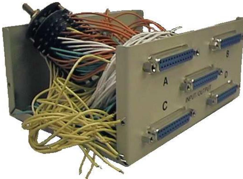
Basically, it is 5 DB25 connectors (yielding a 5-machine WAPERS unit) wired to a big, fat, switch. The next few steps may be easier to do if you first remove the switch and connectors from their mountings in the box.
