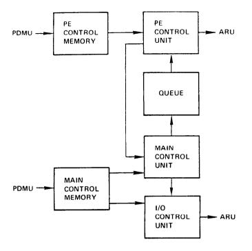
Figure 4 - Block Diagram of Array Control Unit (ACU)
