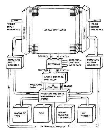
Figure 1 - Block Diagram of Massively Parallel Processor (MPP)
