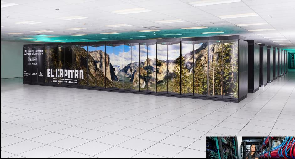
El Capitan supercomputer: 11,039,616 cores, 2.746 Exaflop/s Cost approx. \$600M, 29.6 MW power
