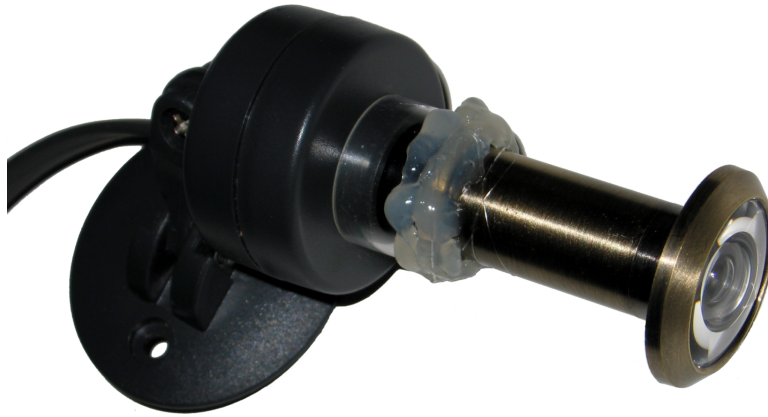
Figure 9: XCam video camera and peephole mounting
