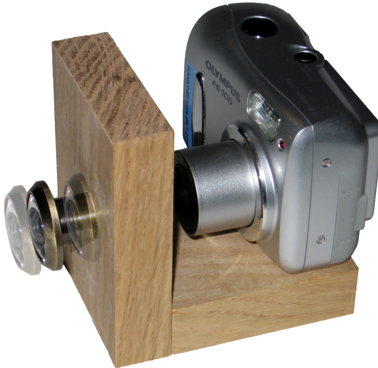
Figure 7: OLYMPUS FE-100 with prototype “sliding” fisheye mount
