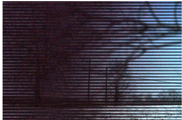
Figure 4. Rolling shutter capture of repeated 1/2000s LCLV events
