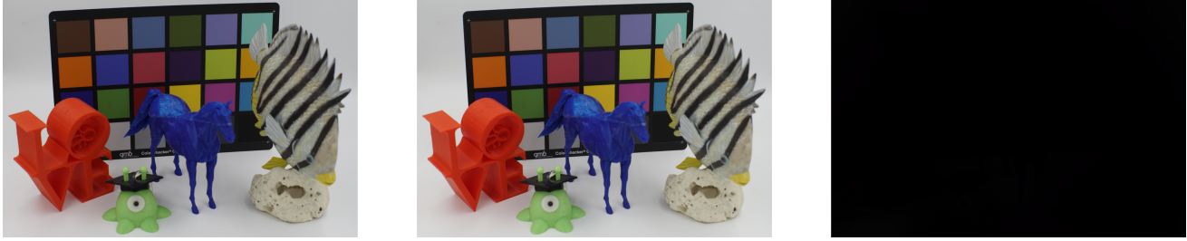
Figure 5. A sample scene captured directly, through the LCLV drive to 0V, and through the LCLV driven to 5V
