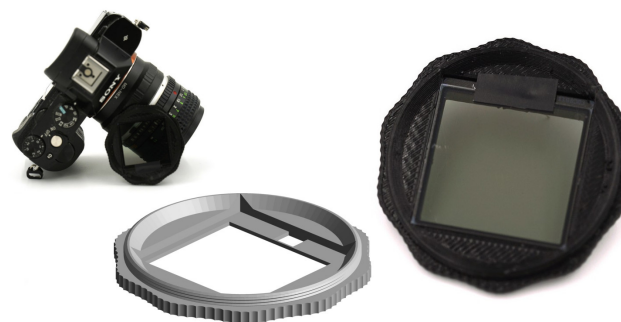
Figure 2. LCLV set in 3D-printed 55mm filter, model and as built
