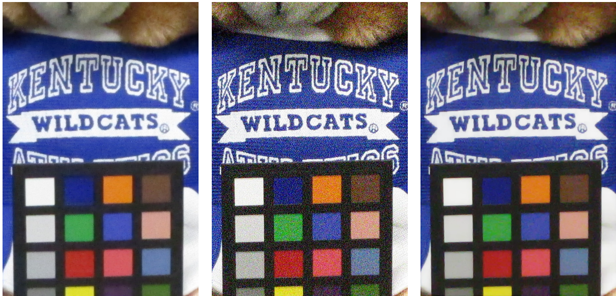
Figure 5. JPEG Crops from Canon A4000 at ISO 1600, 16x ISO 100, and 16x ISO 100 filtered
